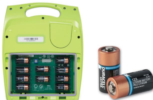
Figure 17: ZOLL AED Plus uses ten 3-volt batteries
