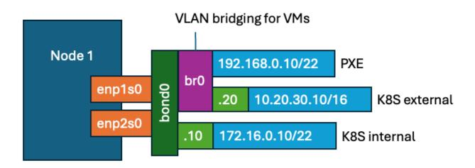
In the example above, we have defined VLAN 20 as a subinterface of **br0** instead of on **bond0**. This configuration allows virtual machines to also run on VLAN 20 without conflict.
