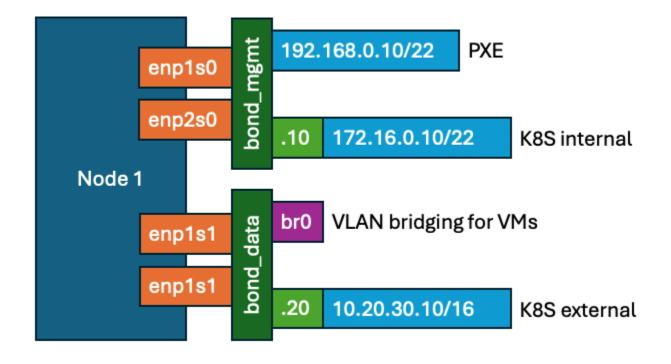
The **br0** bridge interface is used as a master interface for Multus, on top of which Multus can automatically create VLAN interfaces as necessary to place virtual machines onto. The master interface for this scenario must be a bridge interface. It does not work with any other type.
