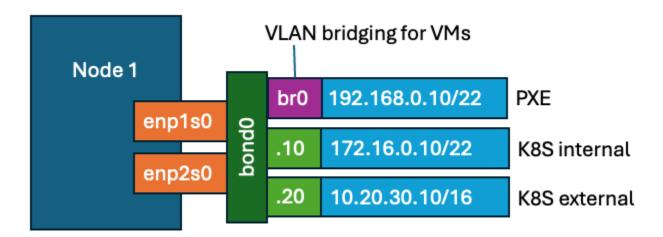
For the setup above, it is assumed that the physical servers (the worker nodes) are connected to the switch as follows:
