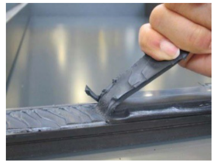
Pull tab to assess adhesion
