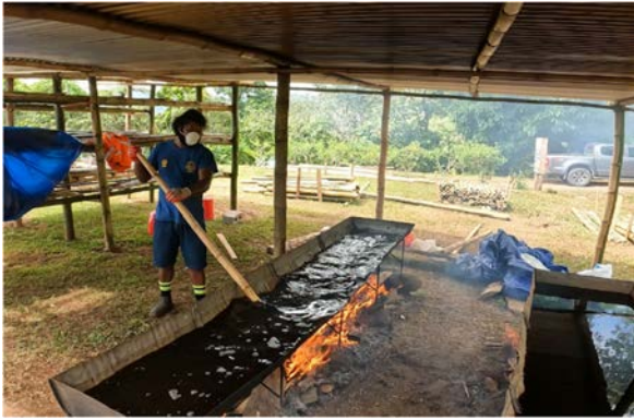
Figure 6-18: Dissolving boron mixture in hot immersion, prior to lacing bamboo into mixture (Pacific Ark)
