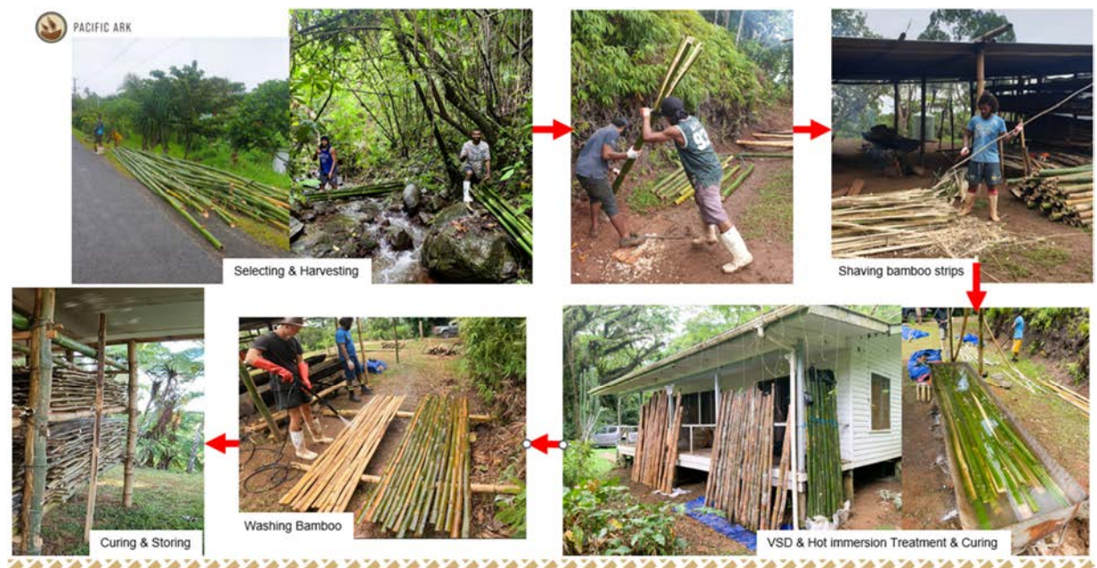
Figure 6-15: Pacific Ark trials from Bamboo Harvesting > Treatment > Prepping > Curing & storing
