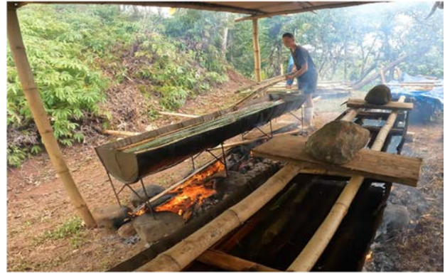
Figure 6-19: Placing bamboo into hot immersion tanks keeping it submerged at all times (Pacific Ark)
