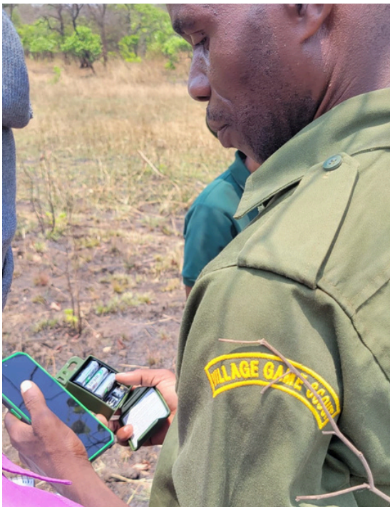
Setting up Song Meter Micro 2 recorders, chosen for their compact design, affordability, and durability. Credit: Wild Survivors.
