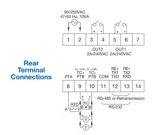
Alarm Functions: Dwell timer Deviation High / Low Alarm Deviation Band High / Low Alarm Process High / Low Alarm Sensor Break Alarm Alarm Mode: Normal, Latching, Hold, Latching / Hold Dwell Timer: 0 - 4553.6 minutes **Data Communications** Interface: RS-232 (1 unit), RS-485 (up to 247 units) Protocol: Modbus Protocol - RTU mode Address: 1-247 Baud Rate: 0.3 - 38.4 Kbits/sec Data Bits: 7 or 8 bits Parity Bit: None, Even or Odd Stop Bit: 1 or 2 bits Communication Buffer: 160 bytes
