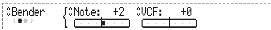
Setting the modulation amounts assigned to the bender via the modulation settings menu.
