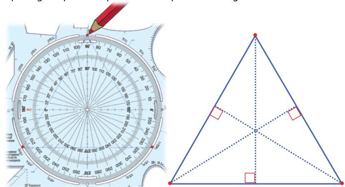
There are many ways to draw larger triangles with Mathomat. This method uses the protractor to mark off points at 90°, 210° and 330° (use the outer hole at 90°'s point).
