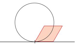
Draw the TGT circle and a tangent to it. Place the 60° rhombus so that its side lines up with the tangent. Draw it in pencil.
