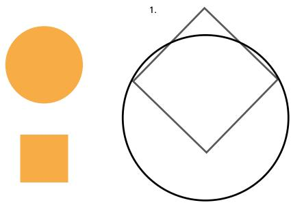
1. Draw Mathomat's TGT circle in ink, rotating it to complete its circle. Place the 25mm square (shape 25) inside and rotate it so that one vertex is outside the circle. The two vertices adjacent to the outside one must both touch a point on the circumference. Draw the square in pencil.
