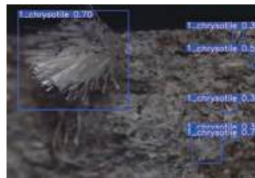
AI-based identification of asbestos fibers using advanced image analysis technology. Example of automated detection of chrysotile (white asbestos).
