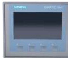
Siemens HMI , a built-in Panel used as a remote desktop display to operate the Siemens S7-1200 PLC .
