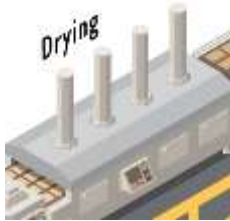
Furnace , equipment used for drying the tiles. Receives commands from the Siemens S7-1200 PLC .
