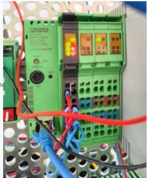
Figure 4 Phoenix Contact PLC ILC 151 ETH
