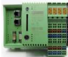
Phoenix Contact ILC 390 PN PLC , a PROFINET controller for the Printer.
