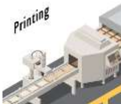
Printer , equipment used for printing the tiles. Receives commands from the Phoenix Contact ILC 390 PN PLC .
