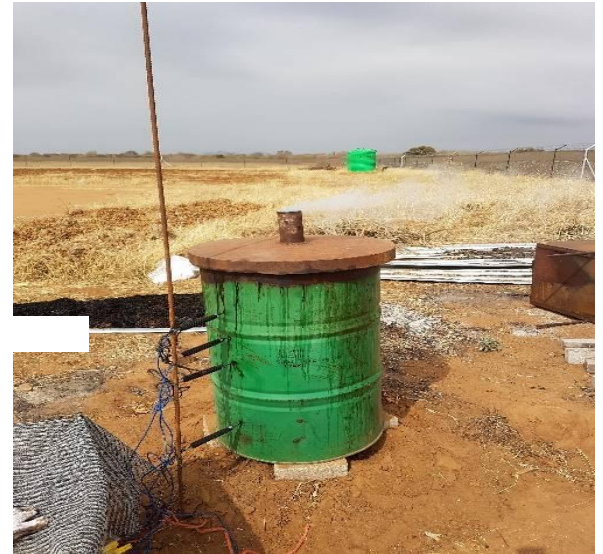
Typical low cost carbonization kiln made of a standard drum in Botswana
