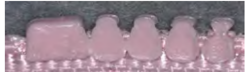
Melted VISLON® elements
