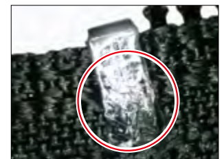
Coil zipper (P-TOP) damage example
