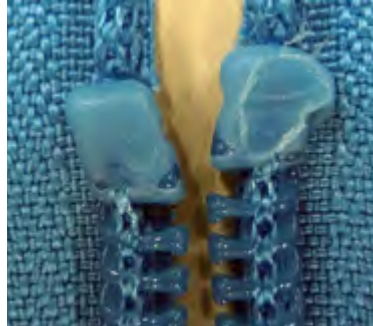
Melted top stop
