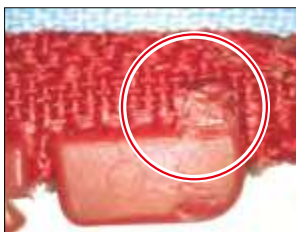
VISLON® (NEWKOB4) damage example
