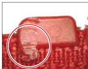
VISLON® (NEWKOB4) damage example
