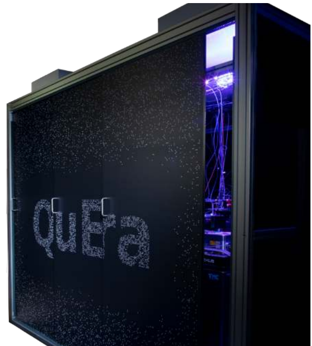
Figure 1.1 The exterior of Aquila, a “field-programmable qubit array” (FPQA) operated as an analog Hamiltonian simulator that implements quantum computations with up to 256 neutral-atom qubits.
