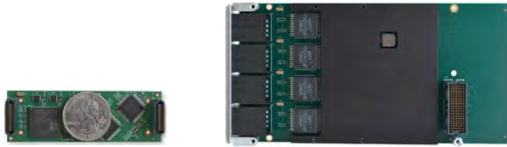
Figure 9: The compact size of QMC is evident when we compare it to the much-larger XMC (VITA 42 and 66) standard.
