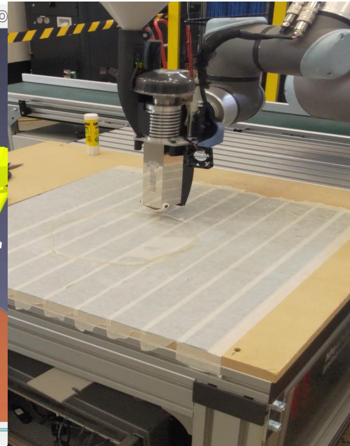
Robotic fabrication WASP 3D Printer - Pellets
