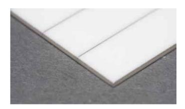
3YSZ is a special partially stabilized zirconia which is used for thin film applications. Among others, it can be used as an ion conductive ceramic membrane for Solid Oxide Fuel Cells (SOFC). This material is characterised by its excellent flexibility, extremely high bending strength and high fracture toughness. Another advantage is that this material can be manufactured in small thicknesses.
