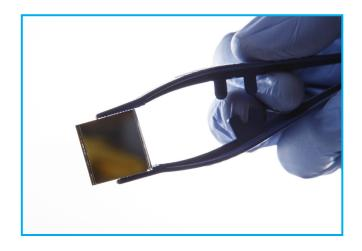
Single crystal substrates are fundamental materials for semiconductor and electronic devices due to their unique physical and electrical properties.
