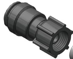
AquaLock connectors utilize a swivel nut with NPS straight threads and a cone seal. This allows the installer to thread onto NPT, NPS, BSP and most 1/2" male threads without tools or thread sealant. Simply thread on, hand tight, for a zero-leak seal.
