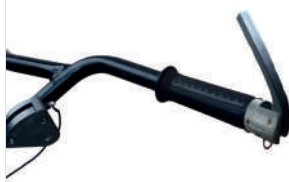
Dead Man Switch Cut Off
