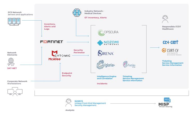
The Valencian Health Department implemented three capture sensors and remote sending of traffic from two smaller hospitals through Opscura technology. This complements the reactive infrastructure made up of firewalls, endpoints, and other barriers that prevent the execution of attacks on the infrastructure.
