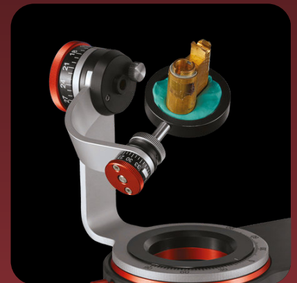
PLASTICINE SUPPORT Plasticine support for mounting deformed, small or oddly shaped items
