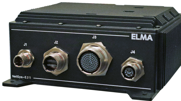
Figure 3: Cisco's Linux-based software router opens the door to custom packaging designs suitable for any deployed space.
