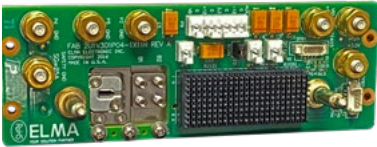
3U 1-slot OpenVPX power and only and VITA 66 aperture
