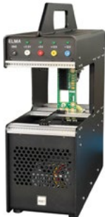
Type 39 CompacFrame Development Platform, 1 - 4 Slot 3U VPX Power and Ground Only Backplane
