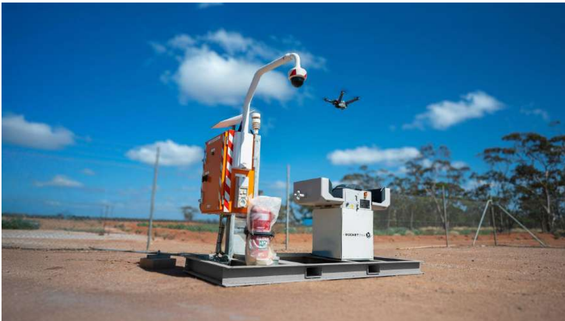
Figure30: DJI Dock incorporated onto a read-to-deploy skid format, minimising installation time and construction setup required for risk-averse environments (Source: RocketDNA )
