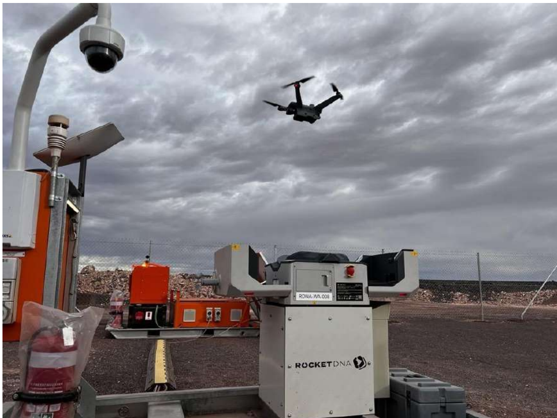
Figure21: Dock 2 landing on-site
