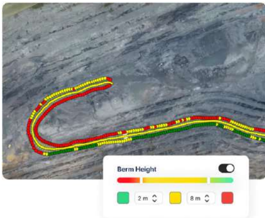
Figure16: Berm height analysis
