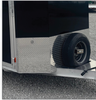
Diamondplate reinforced front rock guard (shown w/optional spare)
