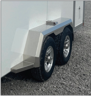
Formed aluminum fenders with multi-function penny lights
