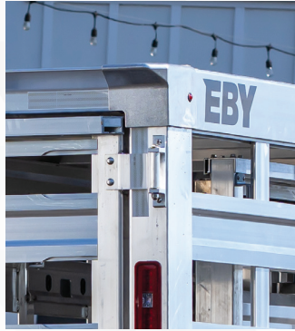
Cast aluminum front and rear corners
