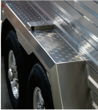
Formed aluminum fenders with multi-function lights
