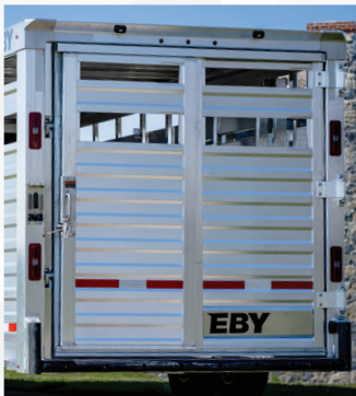
7"x5" Rear frame with slam-shut tailgate
