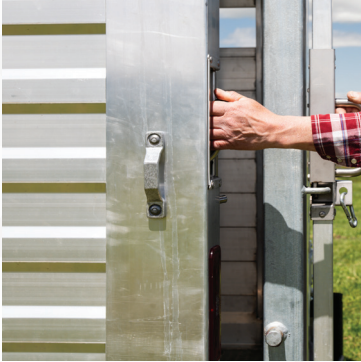
7"x5" Rear frame with slam-shut tailgate
