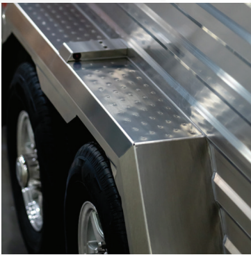
Formed aluminum fenders with multi-function lights
