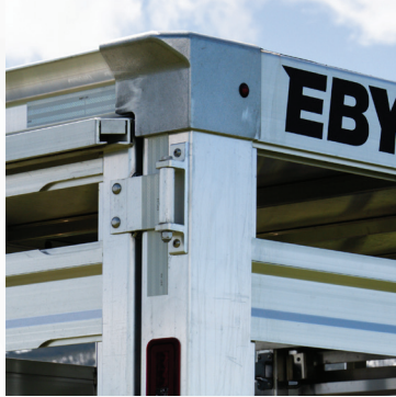
Cast aluminum front and rear corners
