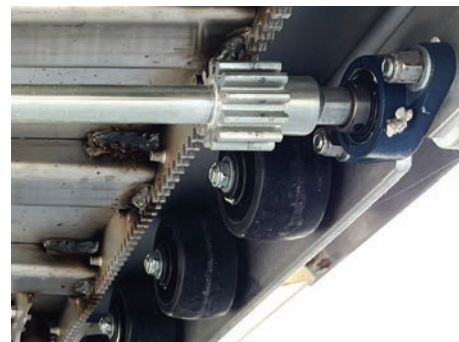
4" roller wheels on the trap doors slide with ease and require little maintenance. Stainless steel trap doors with rack & pinion gearing for long term reliability.
