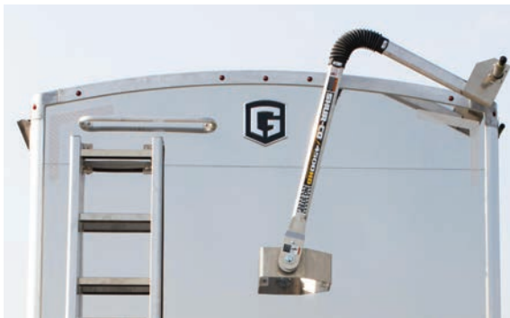
New horizontal seam design on front and rear panels. Cleaner appearance and less panel distortion.
