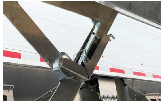
Tarp crank retainer bar stored on curbside dolly leg gusset for emergency access. Easily installed without tools.
