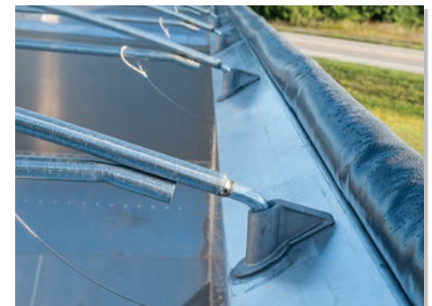
Cast aluminum tarp bow sleeves make it easy to remove and replace tarp bows.
