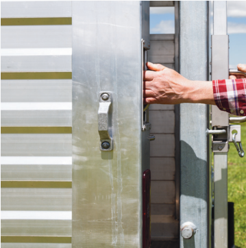
7"x5" Rear frame with slam-shut tailgate
