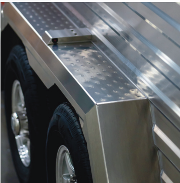
Formed aluminum fenders with multi-function lights
