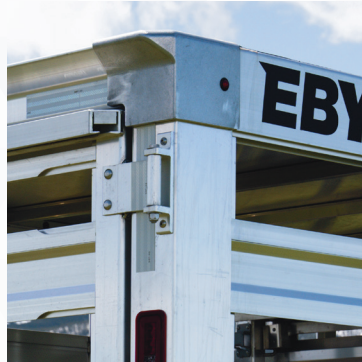
Cast aluminum front and rear corners
