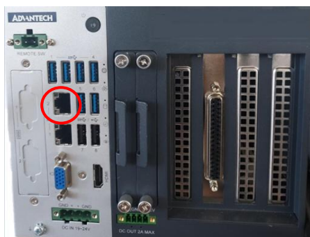
Volta AF-Xplorer™ II workstation Ethernet - Port 2
