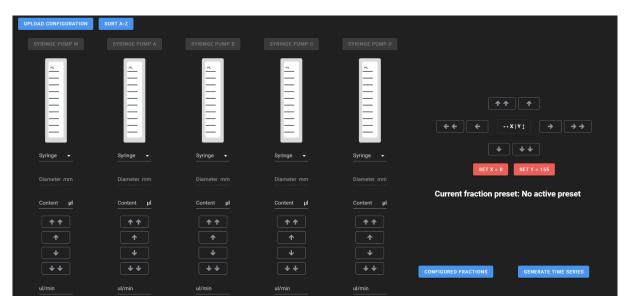
As no preset /fraction layout is activated yet, the fraction collector visualization only shows the movement buttons for the X and Y axis along with their set coordinate buttons.
