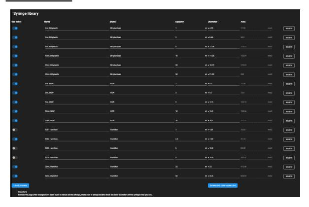
Syringes displayed in the syringe list of the syringe pump configuration module are configured on this page. The blue switch either adds or removes the syringe from the list. Most common syringes are preconfigured, but always double check the diameter of your syringes yourself. Either by datasheets or by a calibration procedure, which we strongly advice doing if highly quantitative results are needed.
