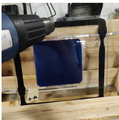
(a) Softening the PIB with the use of a heat gun so the needle can pierce through
