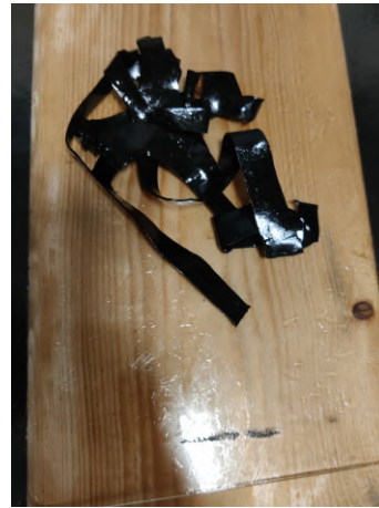
(b) The softened PIB, peeled off in one piece after injecting Mivolt in the module
