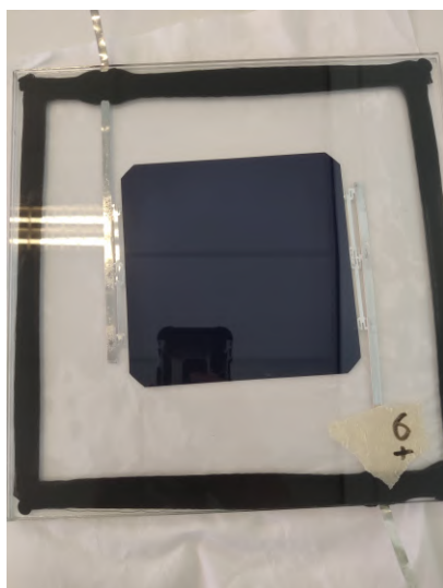
(e) air-filled Module 6 after being submerged in water
