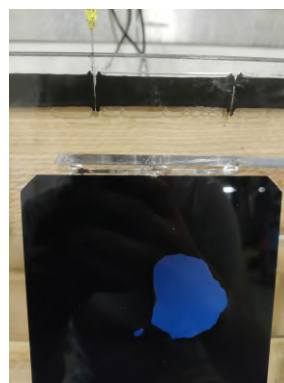
(b) The module directly after liquid injection, with the two required holes and the needle at the top
