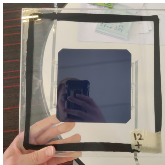
(f) air-filled Module 6 after being submerged in water
