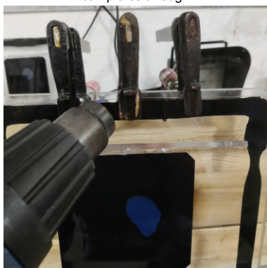
(c) The procedure of closing the module by softening the PIB with a heat gun and by applying pressure with multiple F-clamps for uniformity
