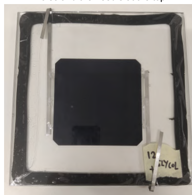
(d) A different module shown for visualisation, with the cell completely submerged after letting it disperse. With the holes used for injection still visible on the right
