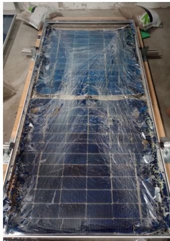
Figure 4. Biosphere PV module design after applying uniform static pressure of 2400Pa.
