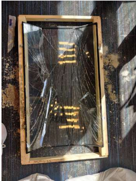
Figure 17 Failed static load test
