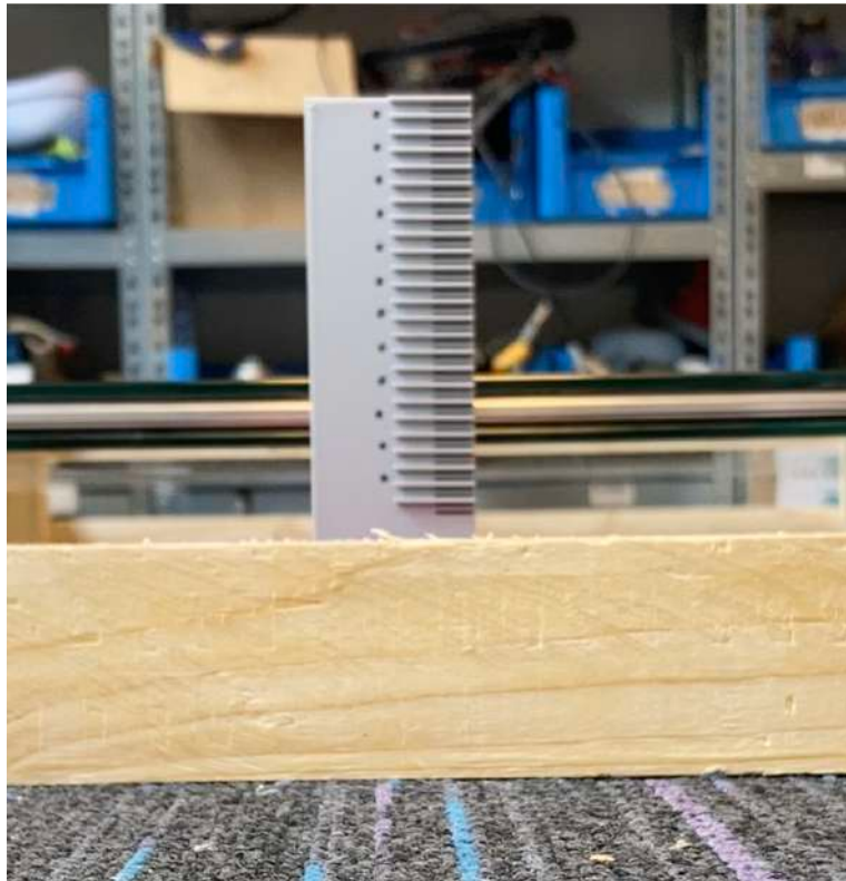
Figure 6 Deflection ruler set-up
