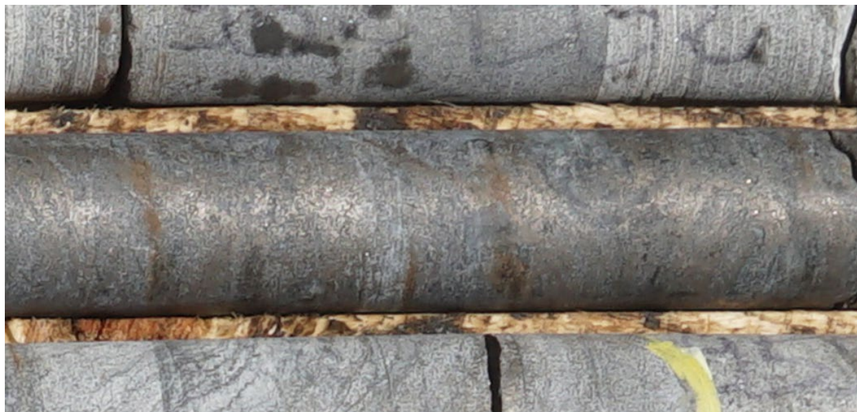
Figure 7: LB-24-29: 954 m, 2.20 m of semi massive, mineralized intercept showing magmatic flows banding of intercalated mineralization and pyroxenite/gabbro magmatic material. It is interpreted as the edge of a larger mineralized system.
