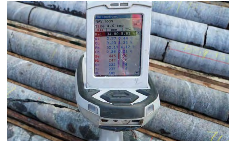
Portable XRF Analysis — Elevated Ni-Cu Readings
