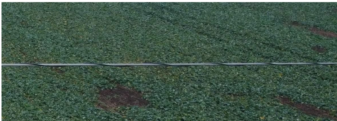
Fig. 3 – Detail of the wrapped conductor
