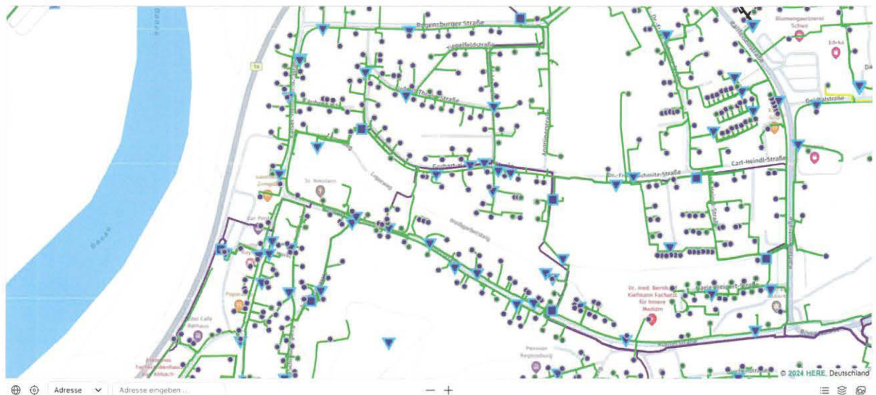
Figure 2. Example of the visualisation of a local distribution network of Bayernwerk Netz based on the digital twin.
