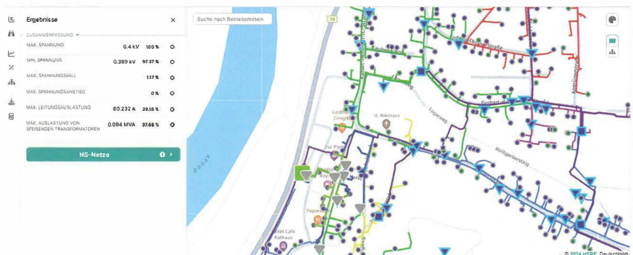
Figure 3. Results view of a secondary digital substation in the digital twin
