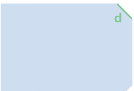
HALF BEVELED d = 0,5 cm thickness = 2,5 or 3 cm
