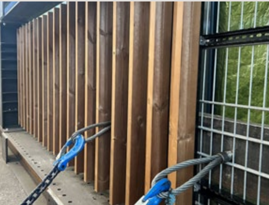
Supports impact loads up to 3.5 t and spanning up to 5.50 m without intermediate support
