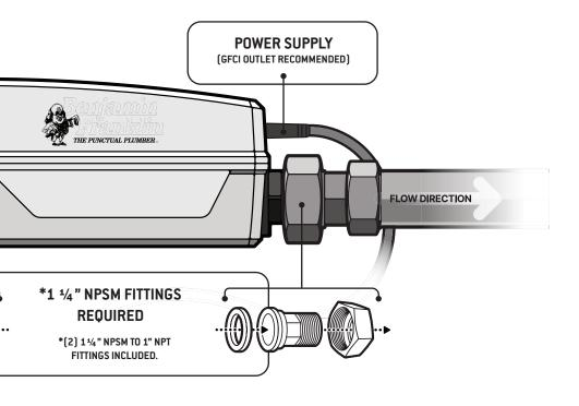
For accurate monitoring and water usage data, your device must be installed <u>BEFORE</u> water heaters, water softeners, whole house filters, etc.
