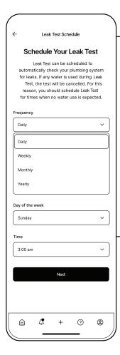
Your device supports periodic testing of your plumbing system's integrity using the Leak Test feature. This feature is particularly useful for detecting small leaks or dripping fixtures. When Leak Test runs, the valve on your device will close automatically and monitor the pressure change in your plumbing system for a period of up to 5 minutes.
