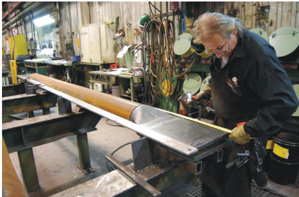
Figure 12 – Fitting of HSC brace assembly. Fitter simultaneously ensures: 1) the HSC connectors are level and in-line 2) the appropriate weld root gap is provided at the joints 3) the overall length of the brace assembly is correct
