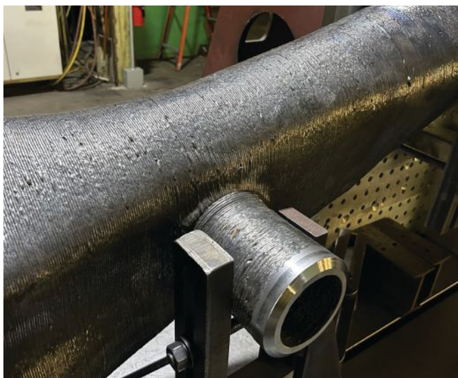
The tree trunk arch bases were left as printed to show one finishing option. The ends of printed shapes (below) were milled smooth to accommodate weld preparations and show another finishing option.
