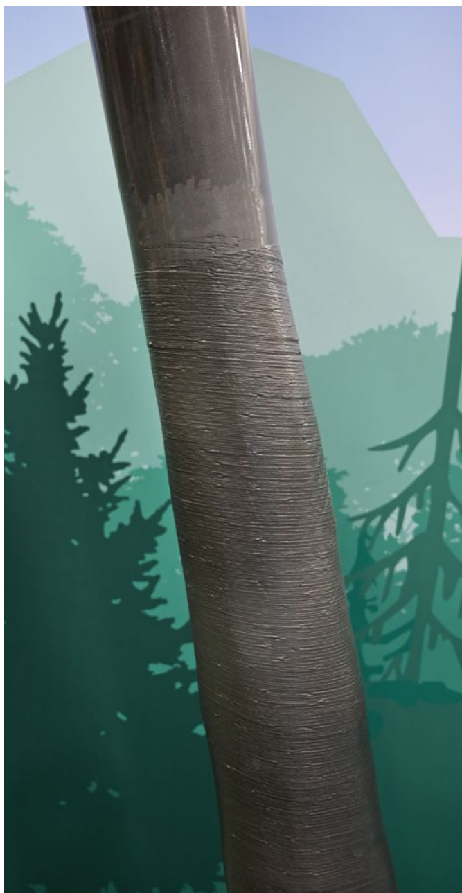
The tree trunk arch bases were left as printed to show one finishing option. The ends of printed shapes (below) were milled smooth to accommodate weld preparations and show another finishing option.
