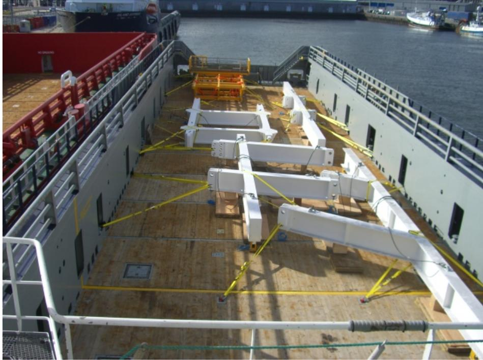
Figure 3 – 5                      Fabricated support frames for new platform facilities
