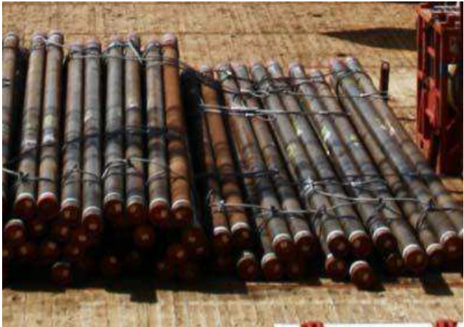
Figure 9 - B - 3 Casing (Dimensions range from 7" to 26")
