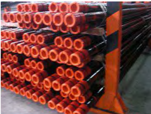
Figure 9 - B - 7 Tubing (Dimensions range from 2 7/8 to 7")
