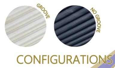
By removing the cord standoff groove, the cords are completely encapsulated in urethane. This protects the core of the belt from hydrolysis and degradation from washdown chemicals, because cord material can wick moisture into the belt body. It also makes the surface easier to clean as dirt and grime cannot cling to the cords.
