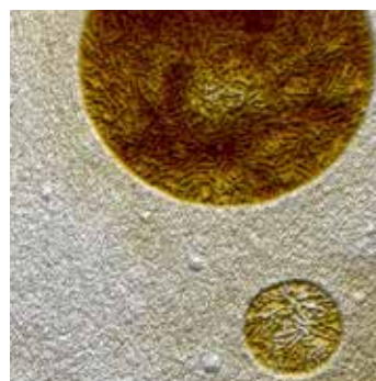
Lamellar structure of LDPE domains embedded in a polystyrene matrix. Image size 1 x 1 μm²
