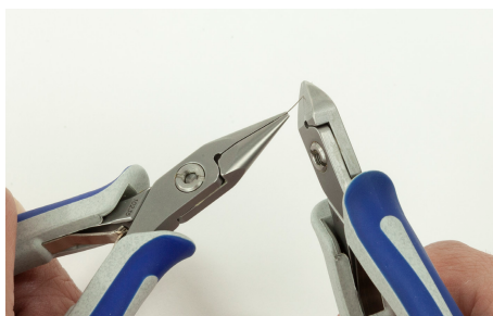
Cut a tip from Pt/Ir wire
