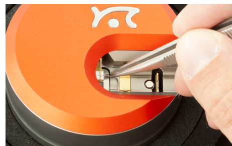
Insert probe into the scan head
